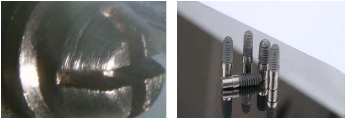
Figure : Cross-grooved anti-rotation notches at the apical end of the intraosseous implant
